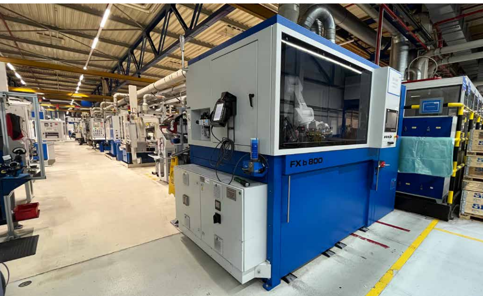
Image on left: The closed cells integrate perfectly into production and significantly reduce noise.
